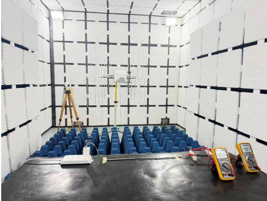
Photograph 3: Set-up for Continuous RF electromagnetic field disturbances
