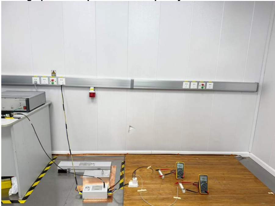
Photograph 4: Set-up for Radio-Frequency Common mode / Conducted Susceptibility
