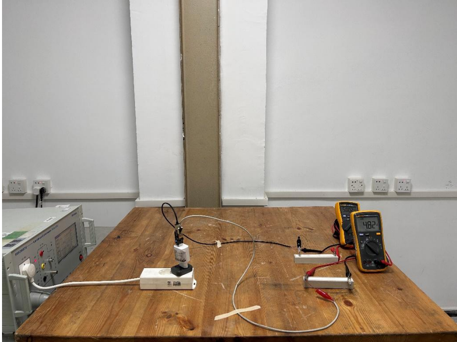
Photograph 8: Set-up for Voltage Dips and Interruptions
