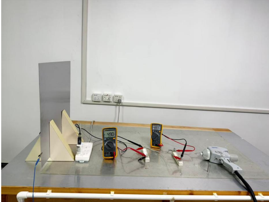
Photograph 7: Set-up for Electrostatic Discharges (ESD)
