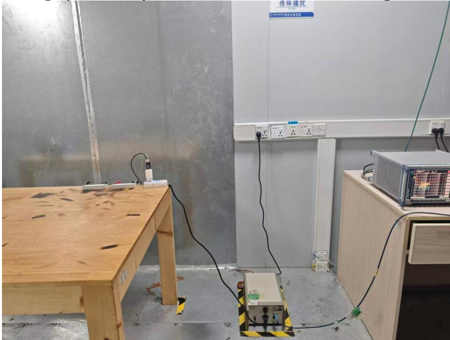
Photograph 2: Set-up for Radiated Emissions (30-1000MHz)
